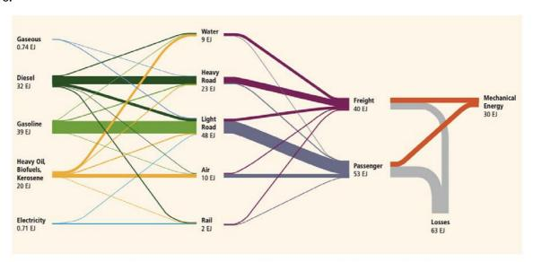
The graph shows final energy consumption of fuels by transport mean in 2009 for freight and passengers. Thermal energy losses account for about two thirds of total energy consumption, with a conversion rate from fuel to kinetic energy of about 32%.
